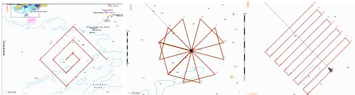
Figure 4: The simulated search paths based on expanding square (left), sector search (middle) and parallel tracks (right) in the absence of current (wind) field. The initial position of search (datum) is  $(50^{\circ}50.0'N, 008^{\circ}50.0'W)$  and the search speed is  $|u| = 10$  kn.
