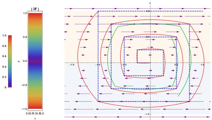
Figure 9: The expanding square model (dotted blue) modified by the piecewise-time-optimal legs (red and green) under the shear (linear) current field  $W = (y, 0)$ . Middle: the current speed (to scale) [24, 25].
