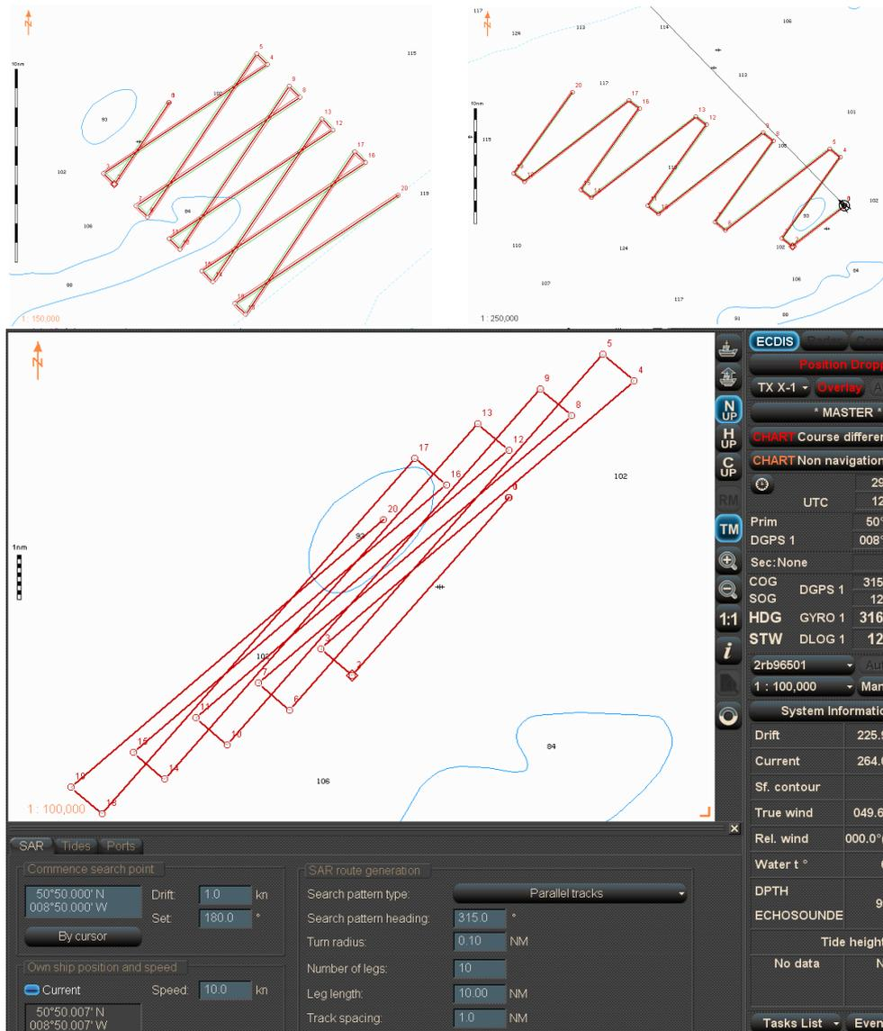
Figure 7: The simulated search paths in the model of parallel tracks, under acting current (wind) field with set of 2.0 kn and drift: 135° (top left), 270° (top right) as well as 1.0 kn and 180° (bottom); the search speed is  $|u| = 10$  kn.
