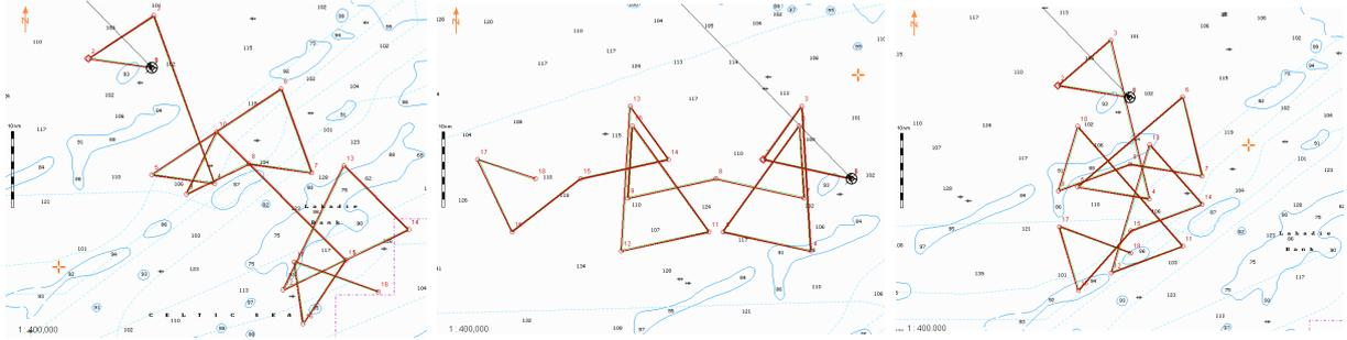
Figure 6: The simulated search paths in the model of sector search, under acting current (wind) field with set of 2.0 kn and drift: 135° (left), 270° (middle) as well as 1.0 kn and 180° (right); the search speed is  $|u| = 10$  kn.
