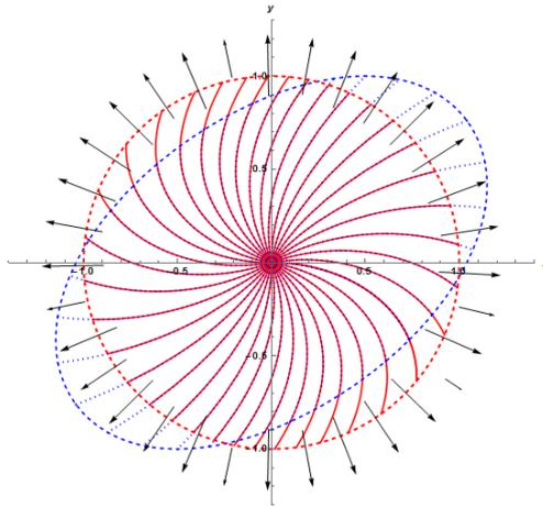
Figure 8: The time-minimal paths (solid red) in a unit disc starting from the origin, with the increments  $\Delta\varphi_0 = 10^\circ$  and the time front ( $t = 1$ , dashed blue), under the linear (shear) wind (or current)  $W = (y, 0)$  [24, 25].
